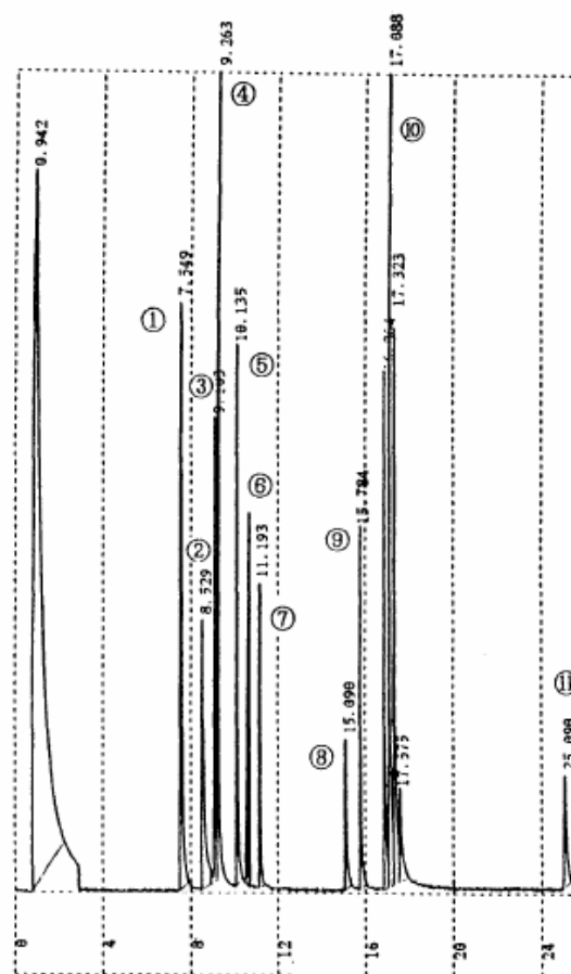
Fig. 2 Typical gas chromatograms of organophosphorus compounds
